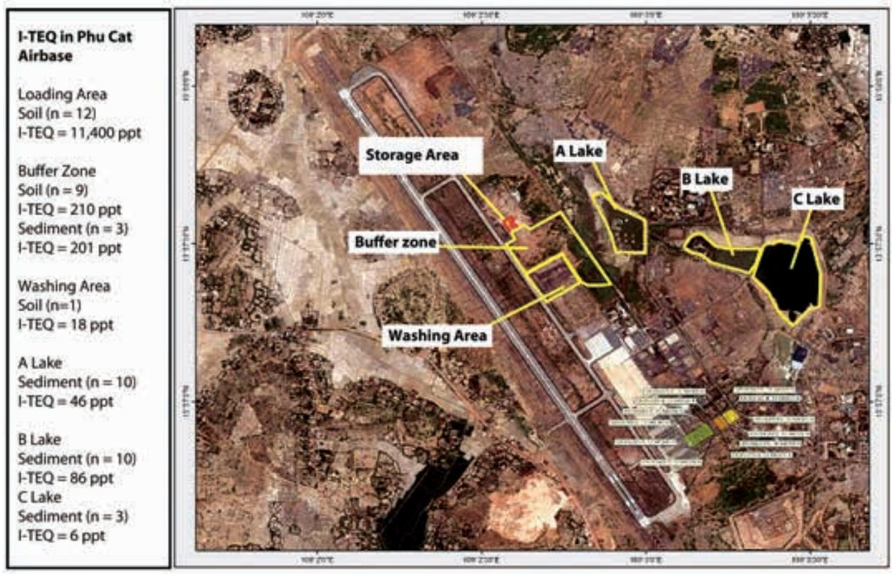
**Fig 4.4. Dioxin concentrations (ppt, TEQ) in soils and sediments from Phu Cat Airbase 1999-2002**
