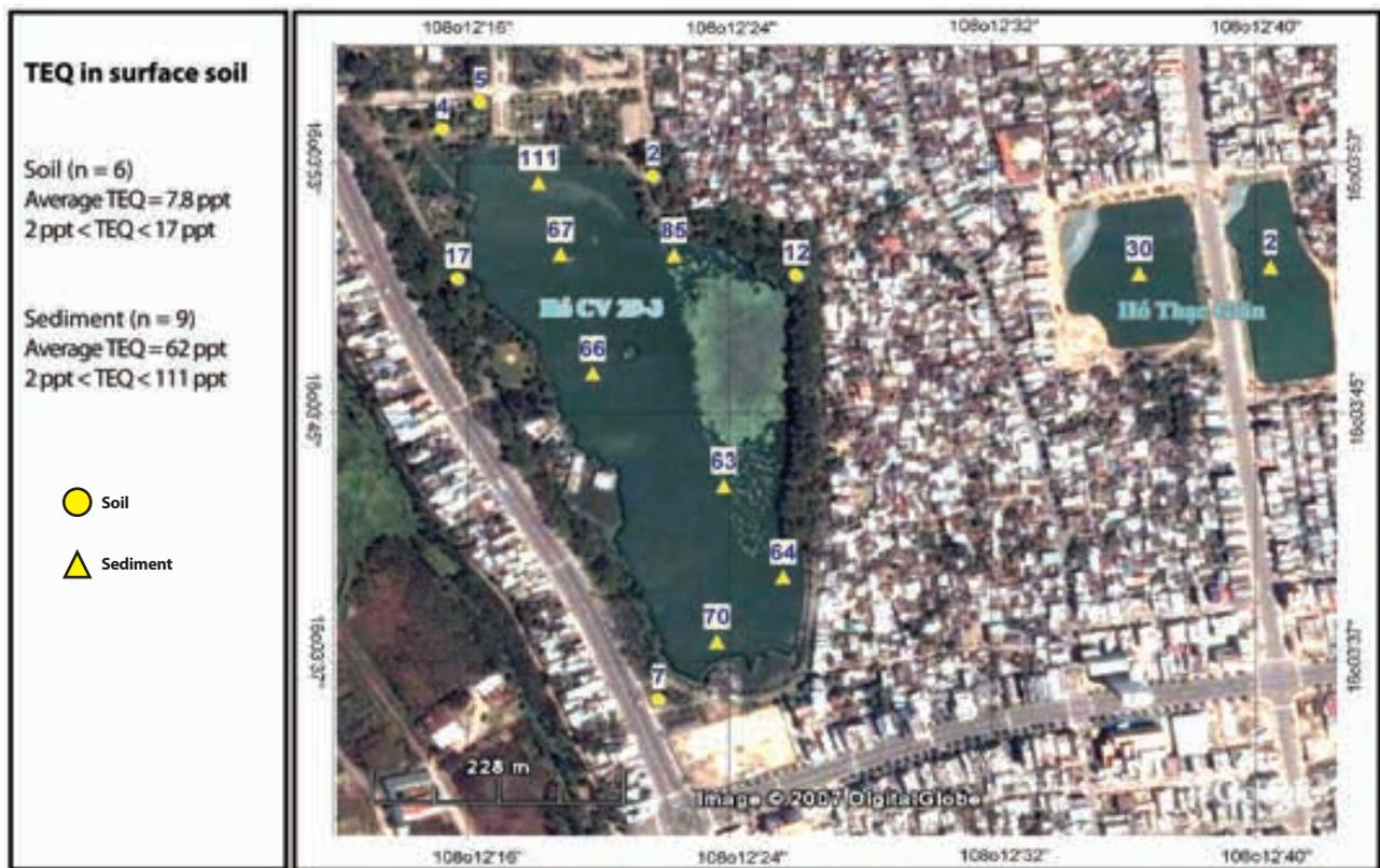
**Fig. 3.6. Dioxin concentrations (TEQ) in soils and sediments from Thac Gian Lake, Da Nang, 2002-2004.**
