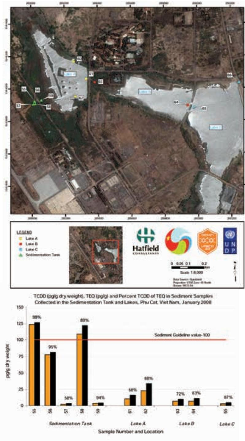
**Fig. 4.11. Sampling locations and dioxin concentrations (ppt, TCDD and TEQ) in sediments from Lakes A, B and C and sedimentation tanks, Phu Cat Airbase, Viet Nam, January 2008.**
